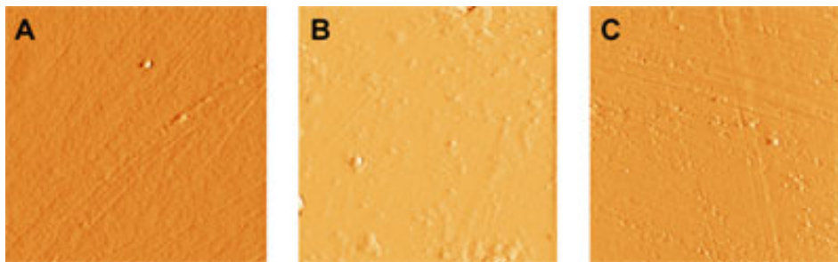
Figure 1. AFM ( 10 \times 0 \mu\text{m}^2 ) error signal of gelatin capsules: (A) untreated; (B) irradiated at 25 kGy by using \gamma -ray; and (C) \beta -ray.
